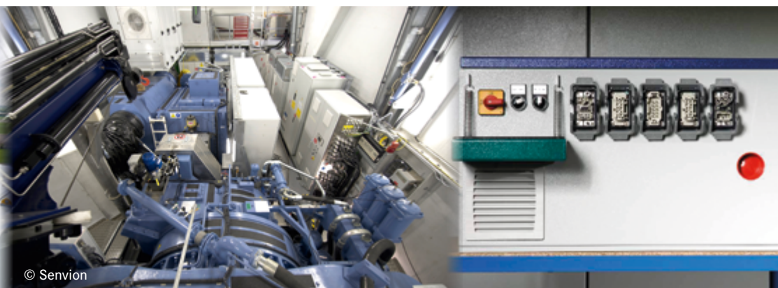
Turbine indoor: pitch system / terminal box / electrical cabinets
