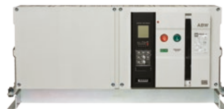
ABW6300 In 6.300 A Icu = 120 kA @ 380 V Ics = 100% Icu
