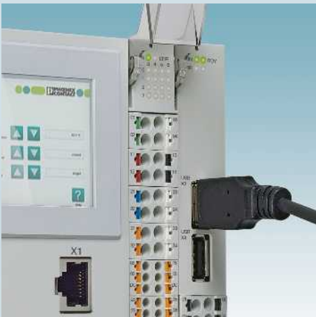
Different front connections for transmitting signals, data, and power
